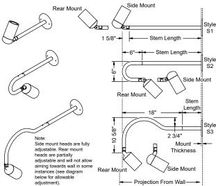
1 5/8" (for Style S1) 6" (for Style S2) 18" (for Style S3) Projection From Wall = Stem Length + Mount Thickness
